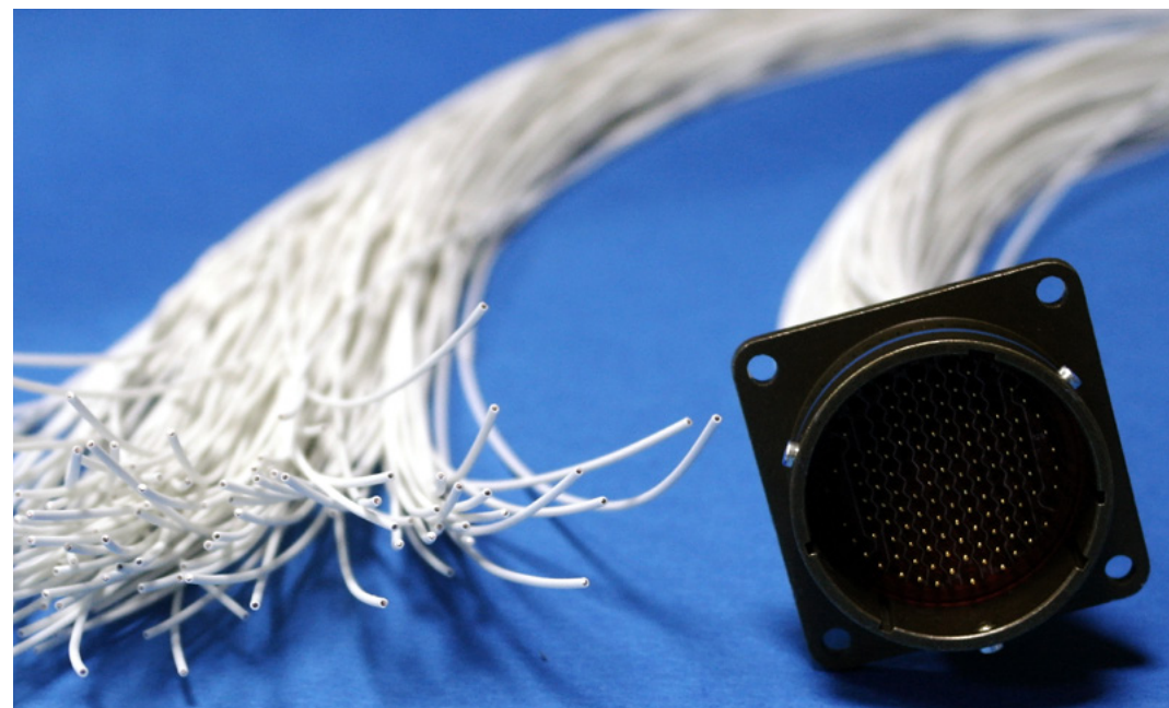
FLYING Camera Cable Connect the camera equipment head portion and flow cables to Left FLAT CABLE, TOP BRACKET FLY_CAM, and RIGHT CAMER I/O B/D
